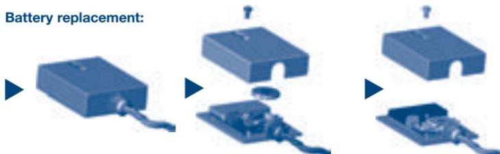
Loosen the screws on the cover (Phillips head screwdriver)
