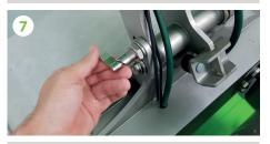
Unlock the feeding hooper through the locker, placing from right to left.
