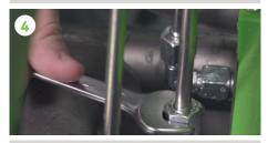
Check the toghtmess of the nuts of the hydraulic pipes.
